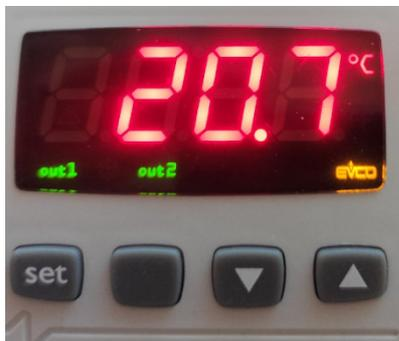
The display shows the temperature measured at the sensor when switched on. The display can be changed to the operating setpoint via parameter P0. The display out1 and out2 shows whether the respective switching contact is active (on = active).
